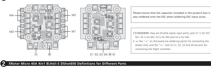
Users only need to connect the throttle control wire, 5V power wire and ground wire of the ESC to the corresponding ports (on peripheral devices like receiver) when a single ESC needs to be programmed.
