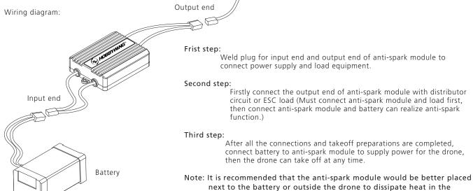
wind. If use anti-spark module for a long time and its shell temparature reaches 110°C, please reduce power to use, otherwise
