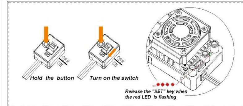
**Note2:** If you don't release the "SET" key as soon as the red LED begins to flash, the ESC will enter the program mode, in such a case, please switch off the ESC and re-calibrate the throttle range again from step A to step D.
