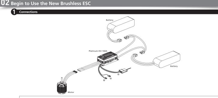
BEC Output Wire (red, brown): Plug the extra BEC output wire (or wire 1) into the special battery channel or any unoccupied channel on the received @ RPM Signal Wire (yellow): Plug this wire (or wire 2) into the RPM input channel on the flybarless system. (User can use the RPM signal wire to provide the RPM signal input when using an external
