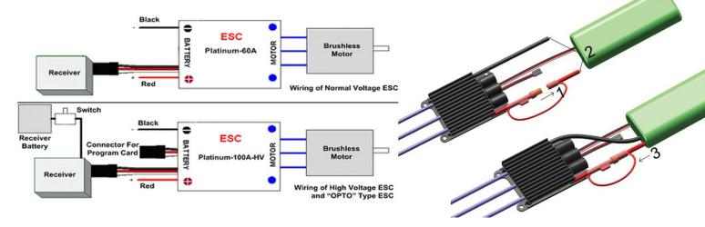
The Platinum-150A-OPTO, Platinum-70A-HV, Platinum-120A-HV, Pentium-80A-HV and Pentium-100A-HV ESC use the new anti-spark structure.
