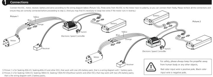
Notes: regarding the SEAKING-130-HV-V3 ESC, the long (White/Red/Black) tricolor wire harness is the throttle wire for connecting to the receiver, the short (White/Red/Black) tricolor
