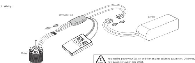
1). Plug the programming cable (on your ESC) into the programming port on the LED program box.
