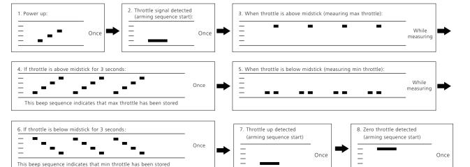
At this point throttle calibration values are stored. You may remove power from the ESC, or just continue running your ESC
