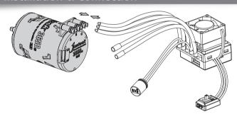
1) Screws used for installation are 3mm in diameter & 5mm in length. Before mounting the motor onto the vehicle, please resize that all the screws are applicable to avoid damaging the motor. In general it's ok to adopt screws which are 3 mm in diameter and less than 8mm in length; the specific length is up to the chassis size.
