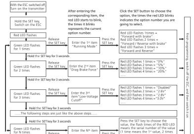
• For easy recognition, the motor beeps at the same time when the LED flashes. When "N" (the number) is equal to/bigger than 5, we use
