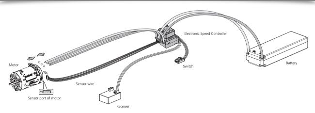
This is an extremely powerful brushless motor system. For your safety and the safety of those around you, we strongly recommend removing your pinion gear before perform calibration and programming functions with this system, and keeping wheels in the air when you turn on the ESC.
