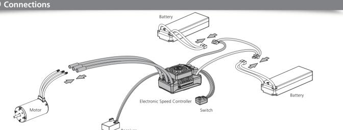
This is an extremely powerful brushless motor system. For your safety and the safety of those around you, we strongly recommend removing the pinion gear before performing calibration and programming functions with this system, and keeping wheels in the air when you turn on the ESC.
