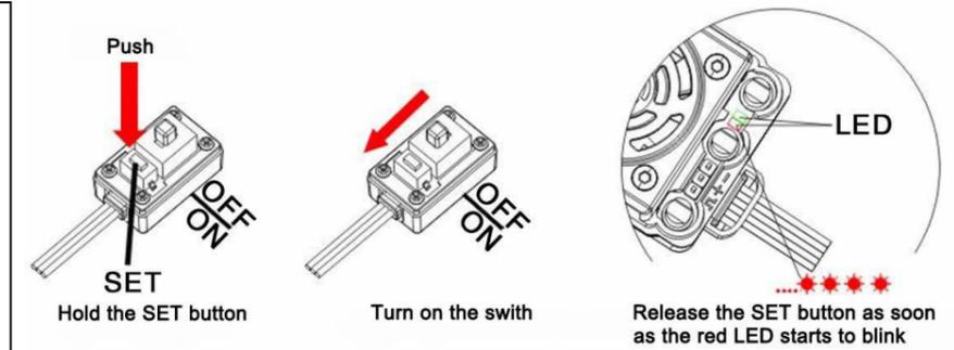
**Note2:** If you don't release the "SET" key as soon as the red LED begins to flash, the ESC will enter the program mode, in such a case, please switch off the ESC and re-calibrate the throttle range again from step A to step D.
