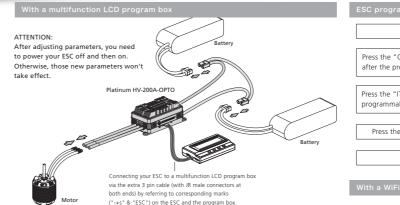
Connect the LCD program box and a battery to your ESC as shown above
